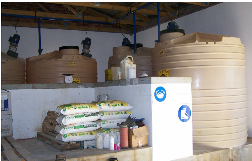
Sophisticated facility for mixing fertilizer materials on the farm. This grower makes up stock tanks and injects each nutrient separately.
